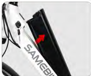
Remove the battery upwards
