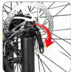
Lock the quick release handle to complete the front wheel installation
