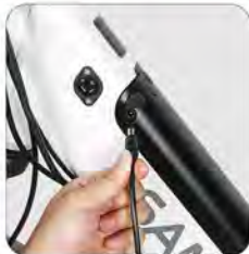
Plug the charger into the power hole
