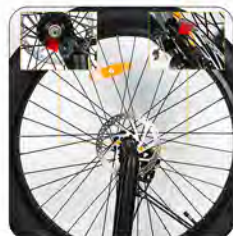
Install the side with the ebiked disc into the direction with the disc brake
