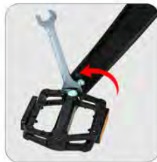
Tighten the left pedal "L" counterclockwise
