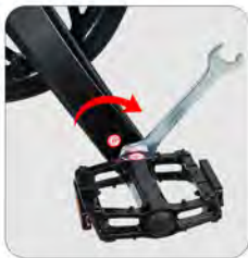
Tighten the right pedal "R" clockwise
