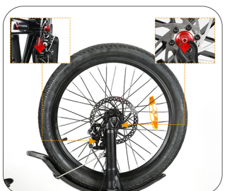
Install the side with the ebiked disc into the direction with the disc brake
