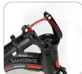
3 Put the riser pipe upright in the direction of the arrow and install it
