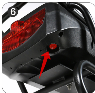
6 switch is located at the bottom of the battery tail. "I" means to turn on the power, and "O" means to turn off the power
